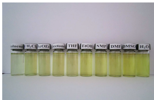
Figure 5. Photograph of dispersion of DE-DHBP-DE in different solvents from left to right: toluene, \text{CH}_2\text{Cl}_2 , AcOEt, acetone, THF, EtOH, NMP, DMF, DMSO and \text{H}_2\text{O} . The concentration is 25 mg/ml in terms of DE-DHBP-DE. [Color figure can be viewed in the online issue, which is available at wileyonlinelibrary.com.]
